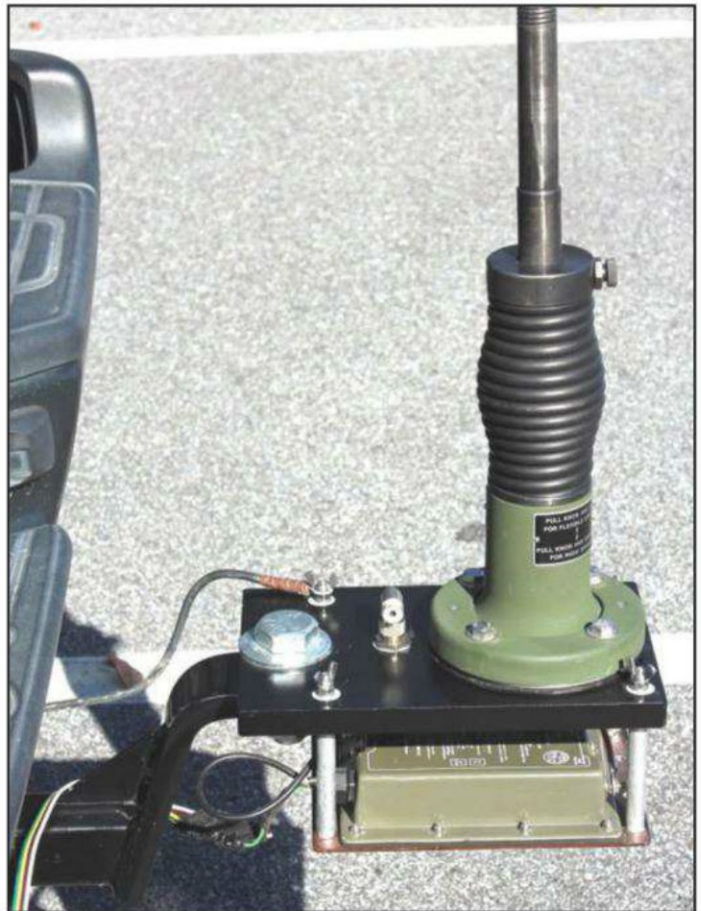
Photo F— Custom AT-1011/U mounting trailer hitch bracket assembly. Additional photos are available online at http://photobucket.com/at1011 and http://photobucket.com/at1011-bonus .
