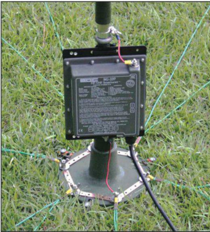
Photo D— Homebrew ground radial anchor ring and eight guys on AT-1011/U flange base. SGC SG-237 tuner is also attached to the base.
