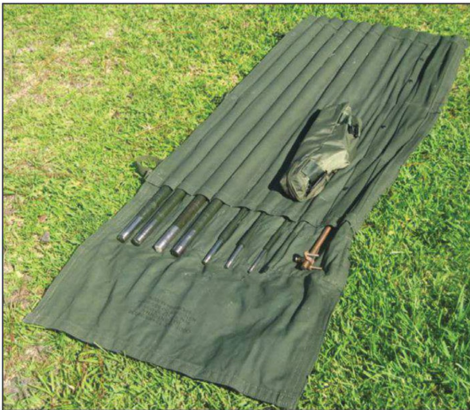
Photo C— AT-1011/U roll-up kit unrolled. Note that the ground rod is not part of the standard kit.
